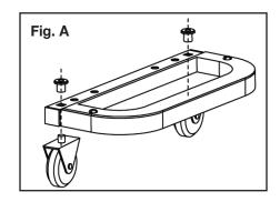
Step 2: To assemble two magnetic tool trays, insert the bolt (No. 10) through the support bar (No. 18), then through the holes on the frame of side tray (No. 4), then through the body frame (No. 2), then add the washer (No. 12) to tighten the nut (No. 11), as shown (Fig. B).
